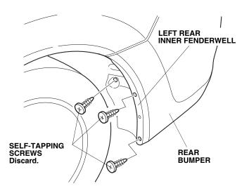
6. Secure the left rear splash guard with three new self-tapping screws, in the order shown below. If there is a gap between the left rear splash guard and the vehicle, loosen the three self-tapping screws and retighten them while pushing in on the splash guard.
