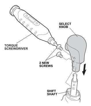
6. Reinstall the shift switch cover on the select knob.
