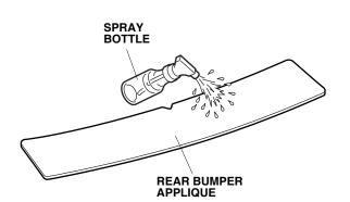
6. Without touching the adhesive side of the rear bumper applique, position it on the rear bumper, and align the v-notch in the rear bumper applique with the center of the trunk lid anchor. Smooth the rear bumper applique along the rear bumper and tape each end at the curved surface.
