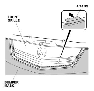
14. Secure four hooks on the bumper mask to the front lower grille.
