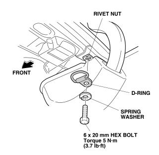
15. Remove the trunk left side trim panel, and repeat steps 5 through 14 to install two T-anchors and a D-ring on the left side of the vehicle.
