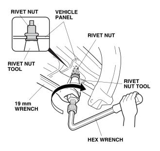
• Remove the tool from the rivet nut by turning the hex wrench counterclockwise.
