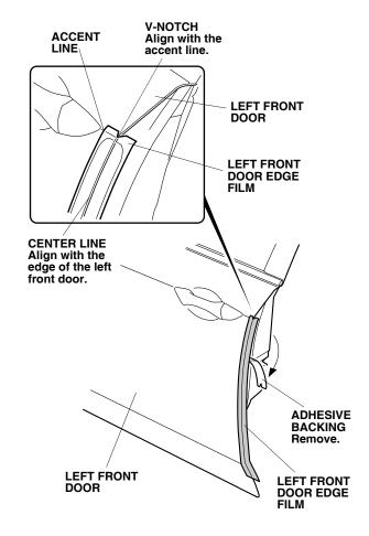
7. Align the center line on the left front door edge film with the edge of the left front door. While applying light pressure, carefully remove the adhesive backing.
