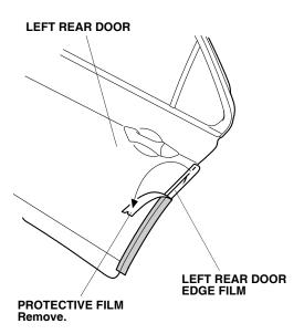
22. Starting from the center and working outward, use your finger and the applicator to fold the left rear door edge film inside the left rear door as shown.
