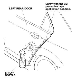
16. Using a spray bottle with the 3M protective tape application solution, spray the outside of the left rear door where the left rear door edge film will attach. Do not spray the inner surface of the left rear door.
