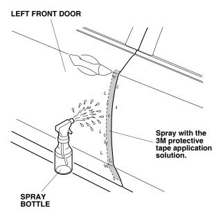
4. Using a spray bottle with the 3M protective tape application solution, spray the outside of the left front door where the left front door edge film will attach. Do not spray the inner surface of the left front door.
