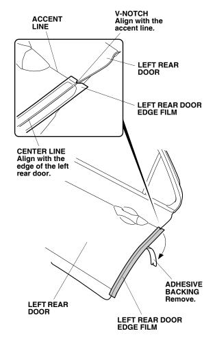
Align the center line on the left rear door edge film with the edge of the left rear door. While applying light pressure, carefully remove the adhesive backing. 20. Starting from the center and working outward, use the applicator to smooth out the left rear door edge film.
