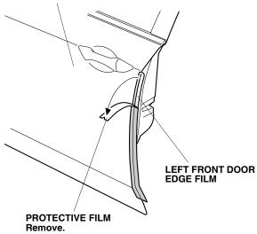
11. Starting from the center and working outward, use your finger and the applicator to fold the left front door edge film inside the left front door as shown.
