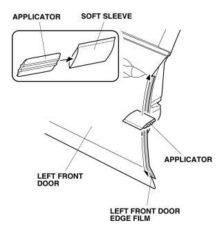
9. Starting from the center and working outward, use the applicator to smooth out the left front door edge film.
