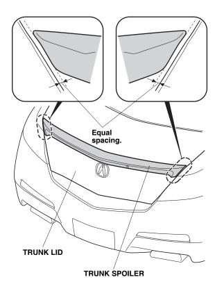
17. Install the trunk spoiler on the trunk lid using the three pins. Install the pins securely by applying pressure on the trunk spoiler with the palm of your hand. Listen carefully for each pin to click into place in its grommet.
