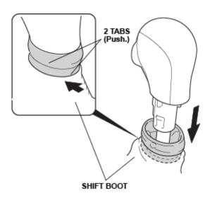
3. Pry out on the bottom of the shift knob cover and remove the cover.
