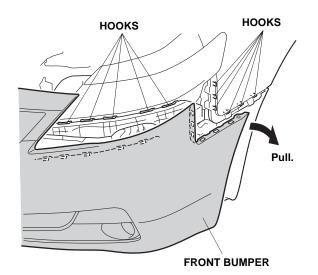
8. With the help of an assistant, remove the front bumper (unplug the five vehicle connectors). Place the front bumper on a blanket so it does not get damaged.
