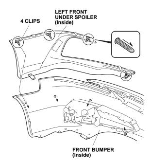
15. Secure the four clip holders onto the four clips.
