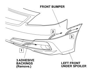
17. Using a rubber roller, apply firm pressure while rolling to set the adhesive.
