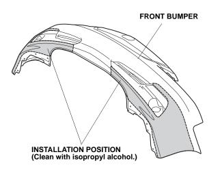
14. Install the left front under spoiler on the front bumper.
