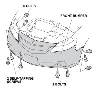
7. On each side, release the 11 hooks, and gently pull the front bumper out from the body.
