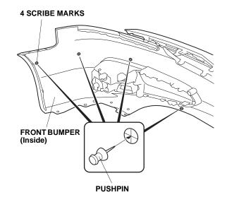
10. While wearing eye protection, drill the four pierced marks using a 3 mm drill bit, then finish with a 10 mm drill bit.
