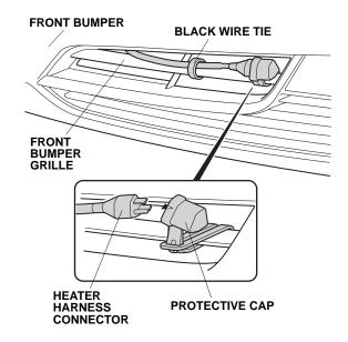
25. Attach the protective cap to the front bumper grille, and plug the heater harness connector into the protective cap.
