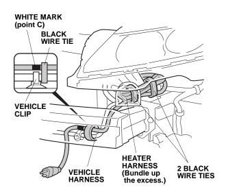
22. Bundle up the excess heater harness, and secure it to the vehicle harness using two black wire ties as shown.
