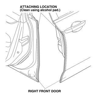
2. Close the front door. Using a spray bottle with 3M protective tape application solution, spray the area where the right front door edge film will attach.
