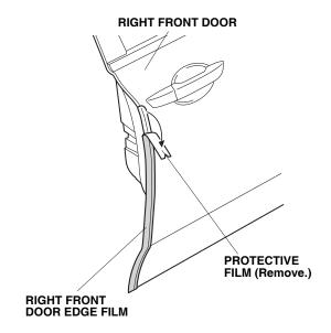
Starting in the middle of the door edge film and working outward, fold the door edge film around the door edge using your fingers. Move your finger in one direction. Attach the film over the seam sealant.
