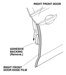
7. Insert the applicator into the soft sleeve. Starting in the middle of the door edge film and working outward, use the applicator to smooth out any bubbles from the film. To avoid lifting the film, move the applicator only in one direction.
