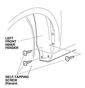
3. Position the left front splash guard on the left front inner fender, and tighten the three self-tapping screws in the order shown.
