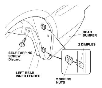
7. Slide two spring nuts over the dimples in the rear bumper.
