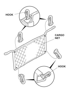
Install the cargo net to the tie down hooks and the anchors in the trunk. The cargo net can be installed in two different positions, vertically or horizontally.
