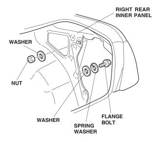
Reinstall all removed parts. Check that all clips are installed securely. 9. Install the anchor to the flange bolt.
