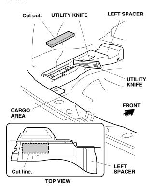
12. Locate the right spacer. Using a utility knife, cut out two sections of the right spacer as shown. Do not damage the vehicle harness under the right spacer.
