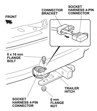
44. Secure the socket harness to the trailer hitch at the black tape using one wire tie.
