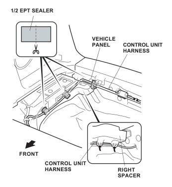
*With Backup Sensors:* Trim the corner of the right spacer to accommodate both wire harnesses.
