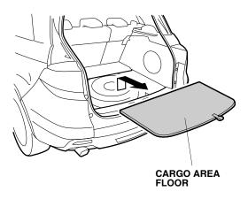
5. Remove the cargo area floor board (four clips).
