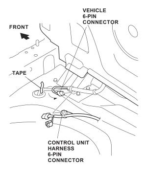
21. Near the 6-pin connector, secure the control unit harness to the vehicle harness with two wire ties.
