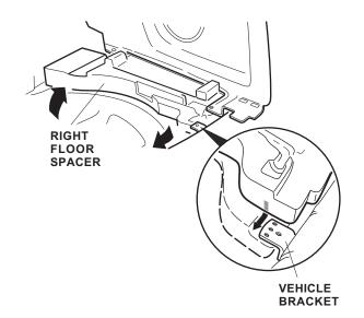
32. Loosely install one 6 x 20 mm flange bolt into the right jack nut.
