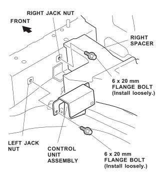
33. Attach the control unit bracket to the vehicle panel using one 6 x 20 mm flange bolt into the left jack nut. Do not tighten the flange bolt at this time.
