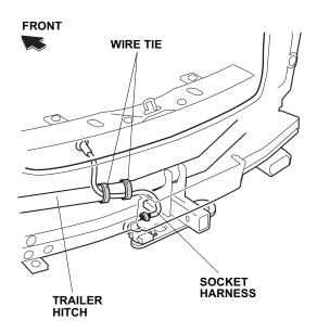
43. Attach the socket harness 4-pin connector to the trailer hitch using the connector bracket, the 6 x16 mm flange bolt and the 6 mm flange nut.
