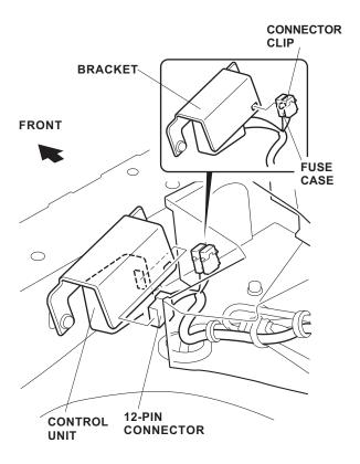
35. Rotate the control unit assembly down onto the right flange bolt. Torque both 6 x 20 mm flange bolts to 4.0 N·m (3.0 lb-ft).
