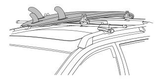
5. Adjust the position of the bases so that the bottom of the surfboard rests on the rubber part of the bases. Tighten all knobs firmly and evenly.
