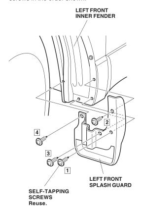
4. Turn the steering wheel all the way clockwise, and repeat steps 2 and 3 to install the right front splash guard.
