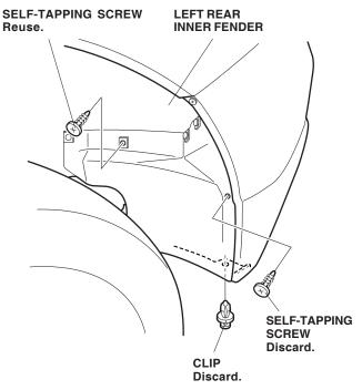
6. Position the left rear splash guard on the rear bumper and inner fender. Install the one clip and one washer screw provided, and the one self-tapping screw removed in step 5.
