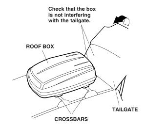
Open the roof box, and align the holes in the plate with the mounting location at the forward crossbar. The plate is located at the front of the base of the roof box.
