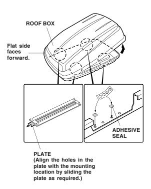
Attach an adhesive seal over each of the four unused mounting holes (two on each side) at the rear of the base of the box. The seals will help prevent water from entering the roof box. Then, remove the roof box from the crossbars. 4. Using isopropyl alcohol on a shop towel, clean four brackets B where the small pads will attach. Remove the adhesive backings from the small pads, and attach them to the brackets B.
