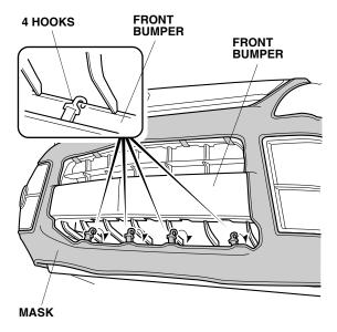
19. Attach the five bottom hooks to the bottom edge of the front bumper.
