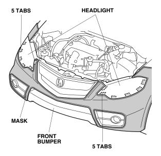
13. Pull the mask back toward the left fenderwell, smooth out any wrinkles, and snap the mask onto the snap-screw.
