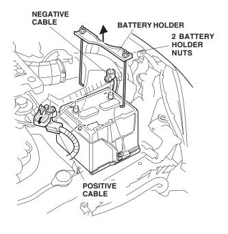
8. Remove the battery cover, battery, and battery box.
