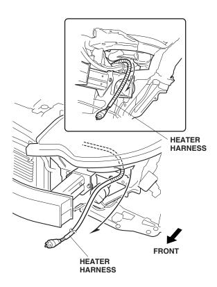
18. Secure the fifth wire tie with clip to the vehicle frame.
