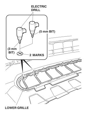
22. Reinstall the front bumper on the vehicle. Secure the heater harness to the front bumper lower grille using two wire ties through the holes drilled in step 21.
