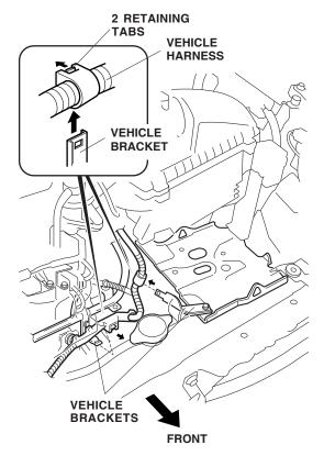
10. Remove the vehicle bracket from the battery tray (one vehicle bolt).
