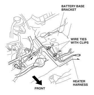
17. Route the heater harness through the front bulkhead opening.
