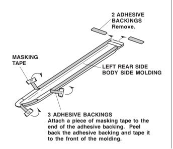
10. Align the front edge of the left rear side molding with the rear template as shown, and attach it using the top edge of the template as a guide.
