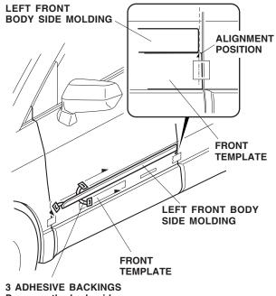
Press on the body side molding firmly with the palm of your hand while removing the adhesive backings.
