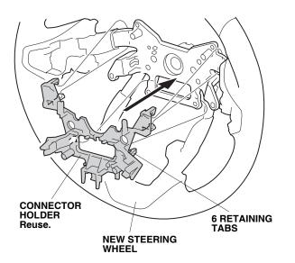
17. Position the steering wheel trim to the new steering wheel, and attach the wiring to the seven retaining tabs.
