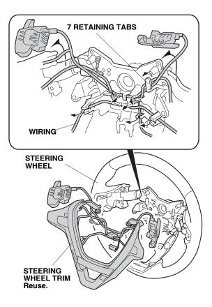
15. Pry up the six retaining tabs, and remove the connector holder from the steering wheel.
