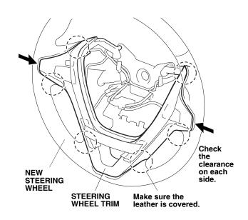
20. Install the two self-tapping screws into the new steering wheel.
