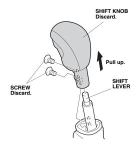
Install the new shift knob using the two new screws. Using a torque screwdriver, torque the screws to 3 N⋅m (18 lb-in). Do not overtighten the screws.
