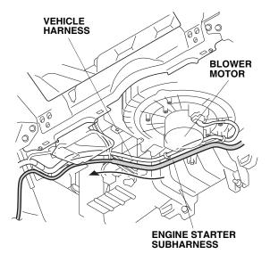
69. Pull the end of the passenger's center console trim to release the one clip shown. Route the engine starter subharness along the vehicle harness to the driver's center console trim opening.
