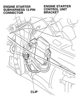
78. Secure the engine starter harness, engine starter subharness, and antenna cable to the vehicle harness with two wire ties as shown. Bundle the excess antenna cable and secure it using one wire tie as shown.
