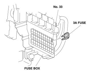
81. Using isopropyl alcohol on a shop towel, clean the area where the fuse label will attach. Attach the 3A ENG STARTER fuse label to the No. 33 slot on the inside of the fuse box lid.
