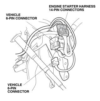
53. Reconnect the vehicle 6-pin connector.
