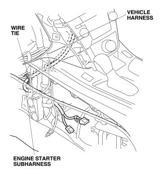
72. Install the clip on the engine starter subharness to the engine starter control unit bracket as shown.
