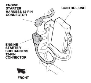
76. Install the engine starter control unit bracket to the vehicle bracket using a flange bolt.
