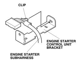
73. Plug the engine starter subharness 28-pin connector into the control unit, and install the control unit bracket. Note the direction of the bracket.
