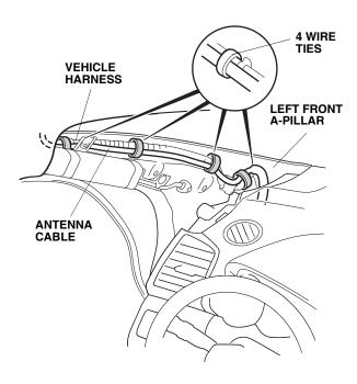
37. Secure the antenna cable to the vehicle harness with one wire tie.
