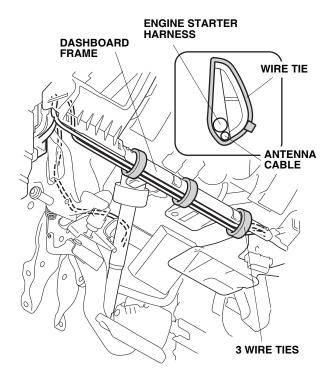
62. Secure the engine starter harness and antenna cable to the vehicle harness with one wire tie.
