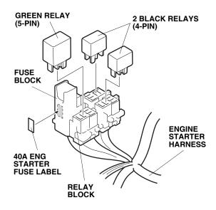
39. Using isopropyl alcohol on a shop towel, clean the fuse block where the fuse label will attach. Attach the 40A ENG STARTER fuse label to the engine starter harness fuse block.
