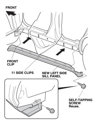
10. Secure the rear portion of the new left side sill panel with the self-tapping screw removed in step 3. Close both doors.
