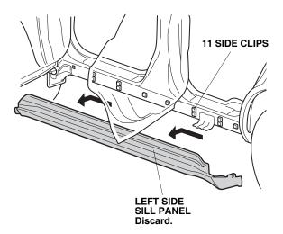
7. Remove the 11 side clips from the body by turning them 45 degrees. Discard the clips.
