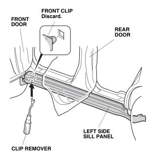
5. Using a clip remover, release the front clip from the back of the left side sill panel.
