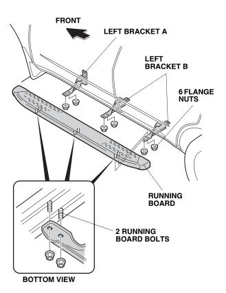
17. Center the running board between the front and the rear fenderwells, then torque all the flange bolts and flange nuts to 27 N·m (20 lbf·ft).
