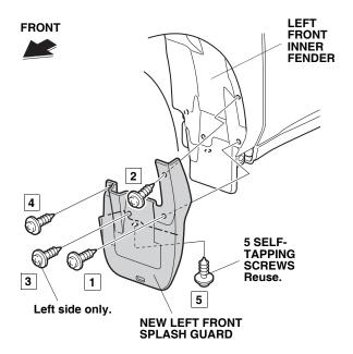
12. While holding the new left front splash guard against the left front inner fender, tighten the self-tapping screws in the order shown. (The right front splash guard uses only four self-tapping screws.)
