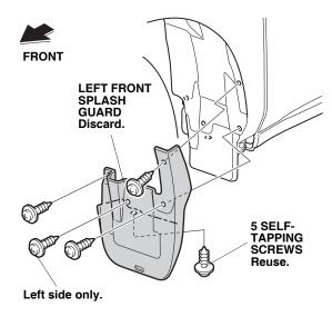
2. Remove the left front splash guard (five self-tapping screws).
