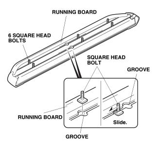
16. Align the six running board bolts to the holes in left brackets A and B, and install the running board with six flange nuts. Do not tighten the flange nuts yet.
