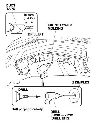
8. While wearing eye protection, drill holes through the centers of the two dimples. First drill with a 3 mm drill bit, and finish with a 7 mm drill bit. Remove any burrs from the edges of the holes with a file.
