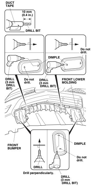
4. While wearing eye protection and holding the front lower molding against the front bumper, use a 3mm drill bit to drill a hole through the center of each of the four dimples shown. Remove any burrs from the edges of the holes with a file.
