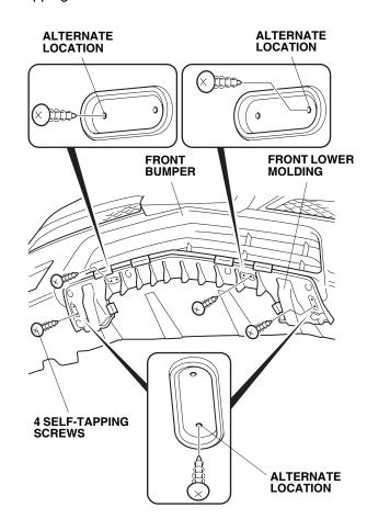
7. Wrap duct tape around a 3 mm and a 7 mm drill bit 10 mm (0.4 in.) from the tip or use a drill stop.
