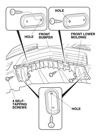
6. Push on the outside edge of the front lower molding to make sure there is no gap.
