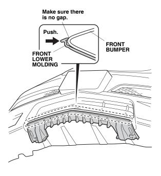
NOTE: If there is a gap to the outside edge of the front lower molding, remove the self-tapping screws and realign the front lower molding. Repeat steps 3 and 4 to drill the four alternate locations, and then reinstall the self-tapping screws in the alternate locations.
