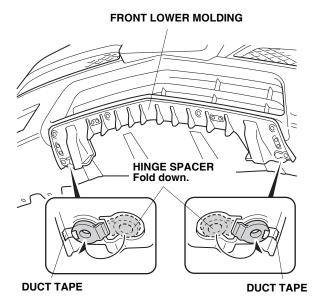
19. Position the front lower trim over the front lower molding, and, install four washers, two 6 x 24 mm special bolts, and two 6 x 40 mm special bolts. Do not tighten the special bolts yet.
