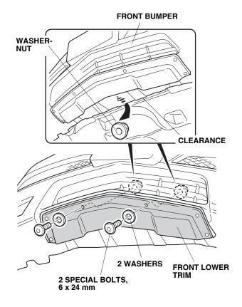
22. Tighten the special bolts in the order shown. Torque the special bolts to 6 to 9 N·m (4.4 to 6.5 lbf·ft).
