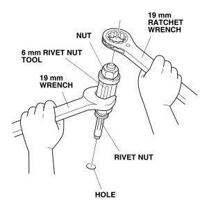
Turn the 19 mm ratchet wrench clockwise while holding the rivet nut tool perpendicular to the work.
