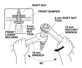
17. Remove the rivet nut tool from the rivet nut by turning the tool body in a counterclockwise direction.
