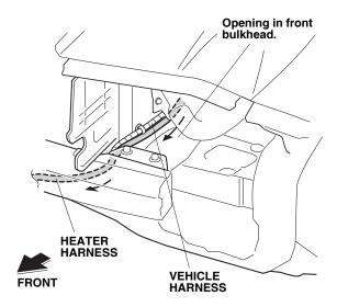
26. Route the heater harness along the bumper beam, and secure it to the vehicle harness using one black wire tie (point D).
