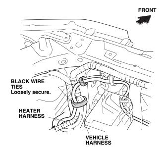
25. Route the heater harness through the opening in the front bulkhead.
