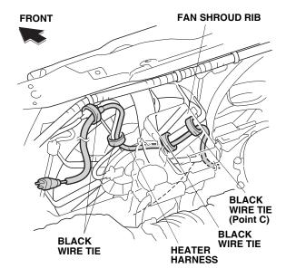
24. Continue routing the heater harness through the engine compartment, and loosely secure it to the vehicle harness with two black wire ties.
