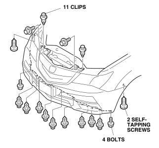
6. With the help of an assistant, unplug the four connectors and remove the front bumper. Set the front bumper on a blanket to prevent damage.
