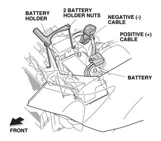
9. Remove the battery and the battery box.
