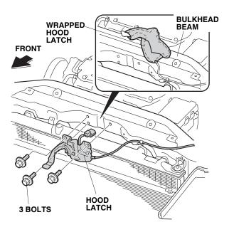
13. Wrap the hood latch in a shop towel, then place the hood latch on the bulkhead beam.
