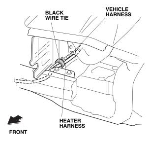
28. Bundle up the excess heater harness, and secure it to the vehicle harness with one black wire tie.
