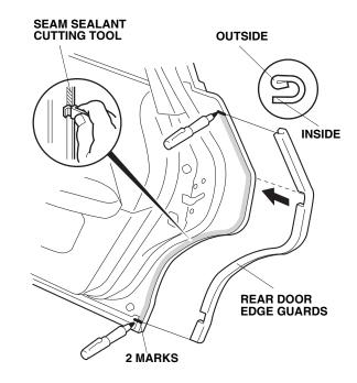
4. Position the cutting edge of the seam sealant cutting tool against the door edge and trim the seam sealant from mark to mark
