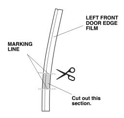
Partially peel back the adhesive backing from the upper part of the left front door edge film. Align the V-notch in the upper part of the door edge film with the end of the character line on the driver's door.
