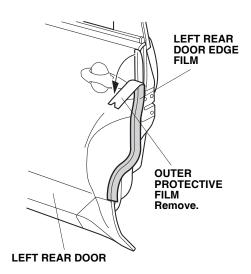
20. Starting in the middle of the door edge film and working outward, use your fingers to fold the door edge film around the edge of the left rear door. Move your fingers in one direction. Attach the door edge film over the seam sealant. Do not trim or damage the seam sealant.
