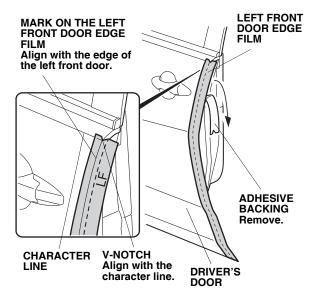
4. Continue to remove the adhesive backing while you align the mark on the left front door edge film with the edge of the driver's door. Go to step 9.
