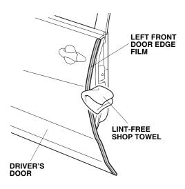
13. Repeat steps 1 thru 12 to install the right front door edge film on the right front door.
