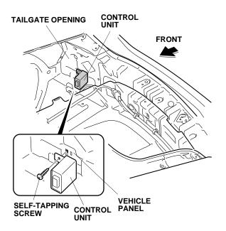
35. Route the control unit harness as shown, and plug the 12-pin connector into the control unit.
