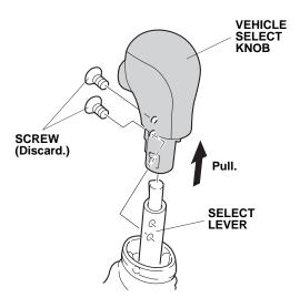
Using a torque screwdriver, install the accessory select knob to the select lever with two screws.
