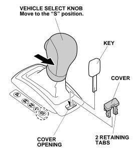
2. Insert a key into the cover opening and move the vehicle select knob to the "S" position.
