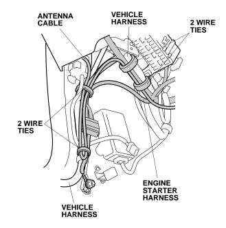
59. Route and secure the engine starter harness to the vehicle harness with two wire ties.
