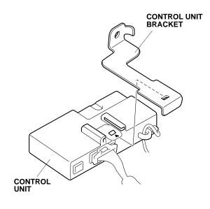
57. Remove the vehicle nut from the vehicle bracket, and secure the control unit bracket to the vehicle bracket with the vehicle nut just removed. Torque the vehicle nut to: 18.7 ~ 24.5 N·m (13.8 ~18.1 lbf·ft).
