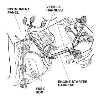
47. Unplug the vehicle 20-pin connector from the fuse box, and plug it into the engine starter harness 20-pin connector. Plug the remaining engine starter harness 20-pin connector into the 20-pin opening in the fuse box.
