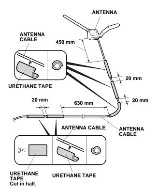
30. Cut one urethane tape in half. Wrap two cut pieces of urethane tape around the antenna cable at the measurements shown.
