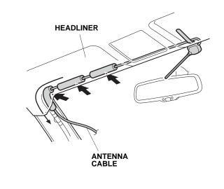
35. Using isopropyl alcohol on a shop towel, thoroughly clean the areas where the urethane tape will attach.
