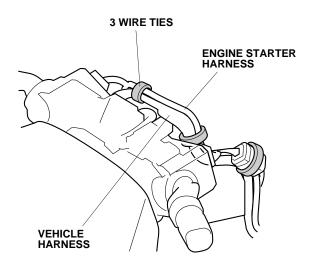
65. Route the engine starter harness to the driver's console side trim opening.
