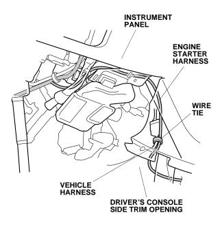
68. Unplug the vehicle 2-pin connector, and plug it into the engine starter harness 2-pin connector. Plug the remaining engine starter harness 2-pin connector into the vehicle 2-pin connector.
