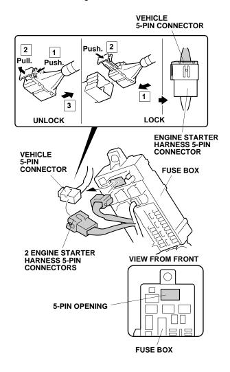
50. Secure the 5-pin connector to the vehicle harness with one wire tie.
