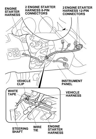
61. Secure the engine starter harness to the vehicle harness with one wire tie.
