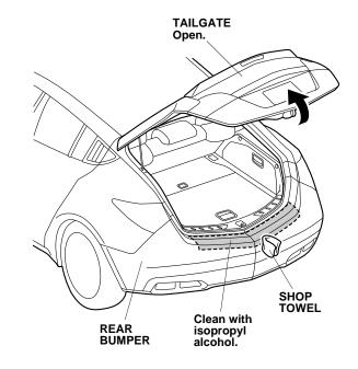
2. Using a spray bottle with the protective tape application solution, spray the area where the rear bumper applique will attach.
