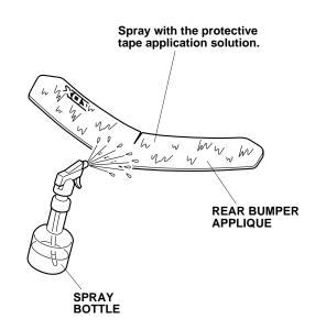
5. Align the center of the rear bumper applique with the character line on the rear bumper.
