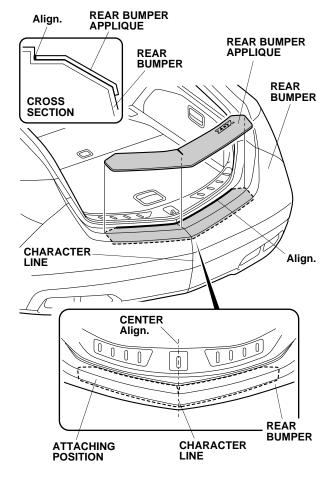
6. Align and attach the rear bumper applique to the rear bumper as shown.
