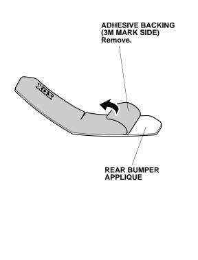
4. Spray the rear bumper applique with the protective tape application solution.
