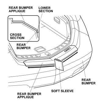
10. Slowly remove the protective film from the rear bumper applique. Remove the film horizontally, do not pull up.
