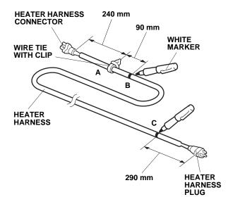
9. Using a tape measure and white marker, measure and mark two points on the heater harness as shown.
