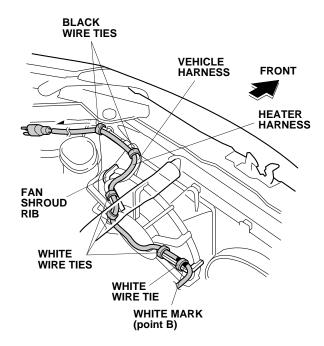
Secure the heater harness to the fan shroud rib and vehicle harness with three white wire ties and two black wire ties. 14. Join two black wire ties as shown.
