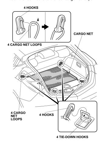
7. Secure the four cargo net hooks to the four tie-down hooks.
