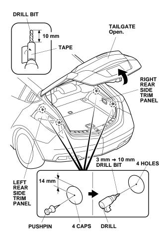
3. While wearing eye protection, drill two holes in the left and two holes in the right rear side trim panels. To prevent damage to the inner panels, wrap tape around the end of each drill bit 10 mm away from the tip. First drill with a 3 mm drill bit, then enlarge the holes with a 10 mm drill bit.
