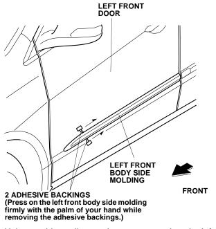
Using a rubber roller, apply pressure against the left front body side molding and roll from one end to the other.
