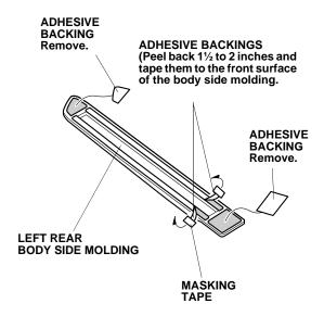
7. Align the left rear body side molding with the template and attach it to the left rear door as shown.
