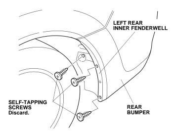
8. Secure the left rear splash guard with three new self-tapping screws, in the order shown below.
