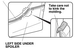
17. Pull the left side under spoiler lightly toward you and check that all five resin brackets fit on the side lower bracket mounting plates securely. If the side under spoiler is loose, repeat the installation procedure.
