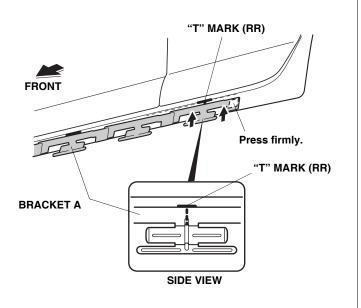
10. Detach the front end of the side lower bracket where you lightly pressed in step 8. Keep holding the end of the bracket. Reposition the top of the bracket to the top of the "T" mark (FR), and press on the front of the bracket firmly to adhere.
