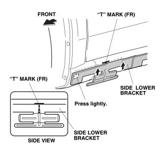
9. Raise the rear of the side lower bracket to contact the top of the "T" mark (RR). Press on the rear of the bracket (where you removed the adhesive backing) firmly to adhere.
