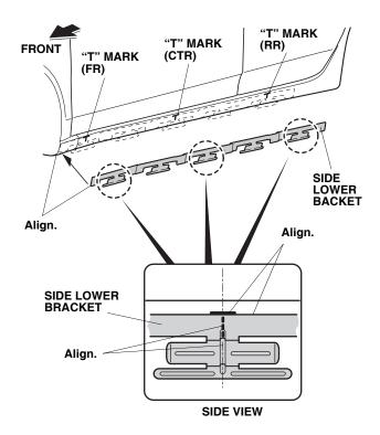
8. Raise the front of the side lower bracket to contact the top of the "T" mark (FR). Press on the front of the bracket (where you removed the adhesive backing) lightly to adhere.
