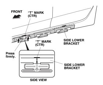
12. Check that the side lower bracket is aligned with the marks. Remove the two adhesive backings from the side lower bracket, starting at the center and working outward while lightly pressing on the bracket.
