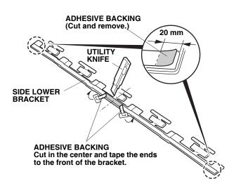
5. Using a utility knife, cut the adhesive backing in the center of the side lower bracket. Attach a piece of masking tape to each of the cut ends, and tape them to the front of the side lower bracket.
