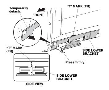
11. Position the top of the side lower bracket to contact the top of the "T" mark (CTR), and press on the bracket to firmly adhere.
