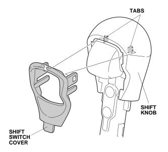
4. Remove the two screws from shift knob, and remove the shift knob by pulling it up.
