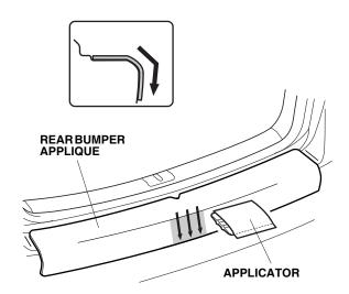
Use the applicator to apply the rear bumper applique to the rounded rear edge on the left side as shown.
