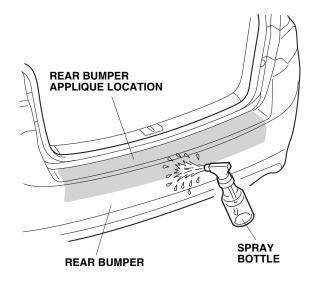
4. Remove the adhesive backing from the rear bumper applique.
