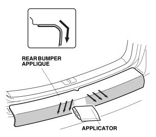
12. Remove the protective film from the rear bumper applique. Slowly pull the protective film back. Avoid pulling it upward.
