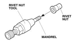
Insert the rivet nut into the hole you just drilled, and install the hex wrench to the rivet nut tool.
