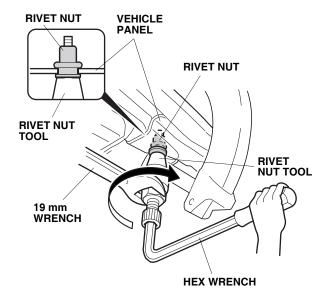
• Remove the tool from the rivet nut by turning the hex wrench counterclockwise.
