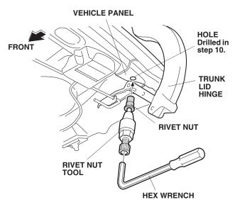
While holding the tool with the hex wrench, use a 19 mm wrench to turn the tool in a clockwise direction until the rivet nut is fully collapsed.
