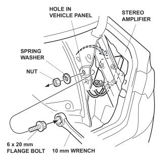
Locate the hole in the vehicle panel. Install one 6 x 20 mm flange bolt through the vehicle panel hole, then install a spring washer and nut. Reinstall the stereo amplifier. 10. In the rear metal shelf, locate the hole near the trunk right hinge arm.
