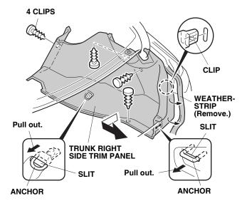
5. On the inside of the trunk right side trim panel, locate the preset mark in the location shown. Using a pushpin, pierce the center of the preset mark.
