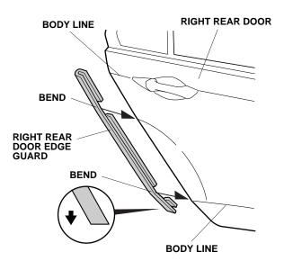
12. Using a felt-tip pen, mark the inside edge of the rear door at the upper and lower ends of the right rear door edge guard.
