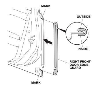
8. Using a rubber mallet, lightly tap around the bend in the right front door edge guard.
