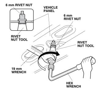
4. Remove the rivet nut tool from the 6 mm rivet nut by turning the hex wrench clockwise.
