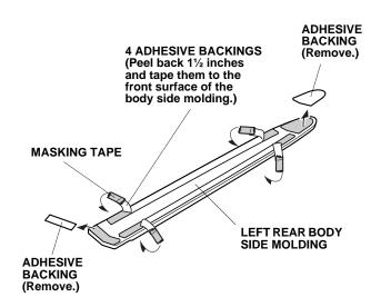
11. Align the edges of the left rear body side molding with the edges of the rear template as shown, and install the left rear body side molding on the left rear door.
