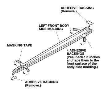
4. Align the edges of the left front body side molding with the edges of the front template as shown, and install the left front body side molding on the left front door.
