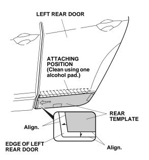
9. Clean the door surface where the left rear body side molding will attach using one alchol pad. Allow the alcohol to dry.
