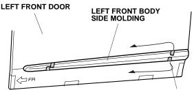
2 ADHESIVE BACKINGS (Press on the left front body side molding firmly with the palm of your hand while removing the adhesive backings.) 6. Using the rubber roller, apply firm pressure while rolling to set the adhesive.
