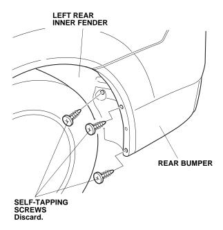
6. Secure the left rear splash guard to the left rear inner fender and rear bumper with three self-tapping screws in the order shown below.
