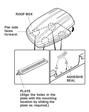
Attach an adhesive seal over each of the four unused mounting holes (two on each side) at the rear of the base of the box. The seals will help prevent water from entering the roof box. Then, remove the roof box from the crossbars. 4. Using isopropyl alcohol on a shop towel, clean four brackets B where the small pads will attach. Remove the adhesive backings from the small pads, and attach them to the brackets B.
