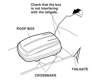
Open the roof box, and align the holes in the plate with the mounting location at the forward crossbar. The plate is located at the front of the base of the roof box.
