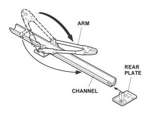
Remove the rubber bumper from the channel, and transfer it to the new location on the channel. Rotate the arm to rest against the rubber bumper. 5. Adjust the front plate to 305 mm from the end of the channel, and retighten the socket bolt.
