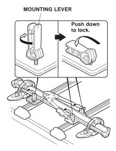
15. Close the locking clamp lever. To deter theft of the bicycle attachment, lock the locking clamp lever with the key.
