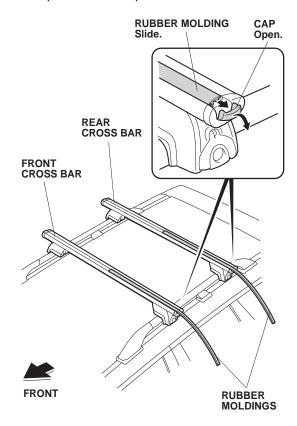
10. Remove the rubber moldings from the T-tracks of the front and rear cross bars. Retain the rubber moldings to be installed later.
