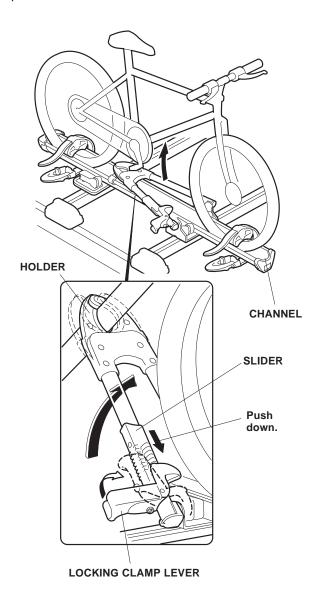
21. Push up the locking clamp lever to secure the bicycle's frame.
