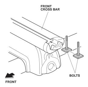
Slide two T-bolts into the front cross bar, and slide one T-bolt into the rear carrier bar. Close the end caps. 12. Position the bicycle attachment over the T-bolts on the carrier bars, and install the mounting levers removed in step 8. Do not tighten or lock the mounting levers at this time.
