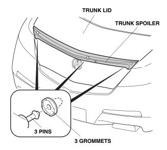
18. Open the trunk lid. Use a flashlight to confirm that the three pins are seated properly in their grommets.
