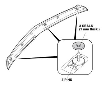
15. Align the pins in each slot with the marks shown.
