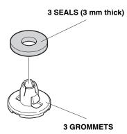
12. Install the three grommets into the trunk lid in the holes shown.
