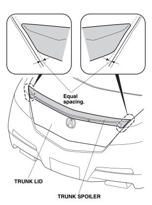
17. Install the trunk spoiler on the trunk lid using the three pins. Install the pins securely by applying pressure on the trunk spoiler with the palm of your hand. Listen carefully for each pin to click into place in its grommet.
