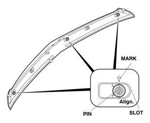
Center the spoiler on the trunk lid, and check the distance on each side.
