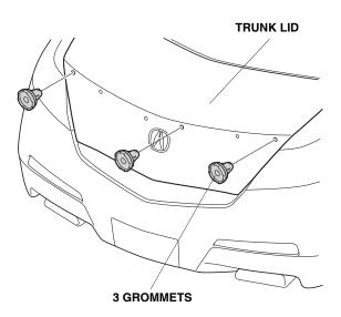
13. Install three pins on the trunk spoiler in the slots shown.
