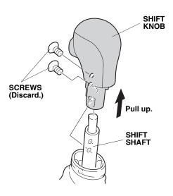
5. Install the new select knob using the two new screws. Using a torque screwdriver, torque the screws to 1.57 N·m (14 lb-in). Do not overtighten the screws.
