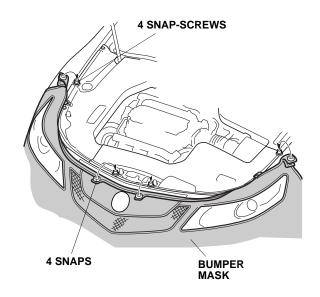
18. Attach the four hooks along the bottom of the mask to the bumper in the areas shown.
