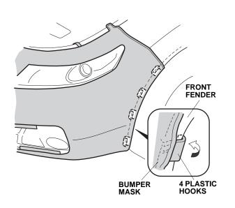
15. Attach the plastic hooks to the other fender the same way.
