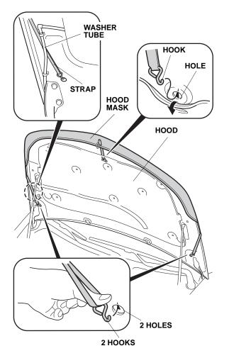
4. Attach the three hooks to the positions shown.
