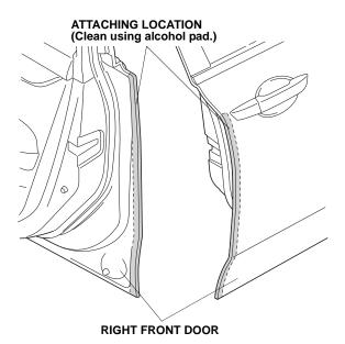
Close the front door. Using a spray bottle with 3M protective tape application solution, spray the area where the right front door edge film will attach.
