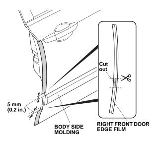
Continue to remove the adhesive backing while you align the centerline on the door edge film with the edge of the door.
