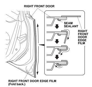
10. Using a lint-free shop towel, wipe up water from the right front door edge film. Allow the right front door edge film to dry thoroughly.
